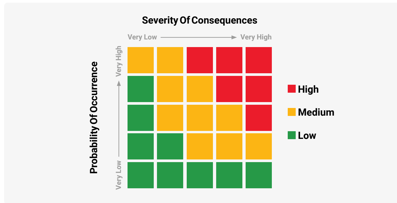
Generic structure of a 5x5 risk matrix system, with colour-coded low, medium and high levels of threat for associated risks.
